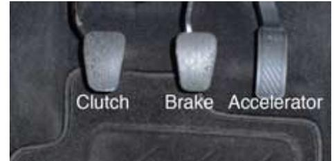
A-B-C When the Accelerator or Gas pedal is depressed (using your right foot) fuel is supplied to the engine. The further down you depress the pedal the more power will be produced from the engine, when the foot is removed off the pedal no more fuel is supplied and the engine power decreases. The engine will not completely stop if the pressure on the pedal is zero, the engine has computers on board to allow smooth running at low engine speeds.
